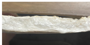
Figure 10. Mulberry fibre artificial leather paste - before applying lacquer.
