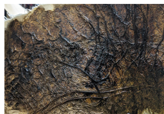
Figure 13. Mulberry fibre artificial leather sheet - after applying lacquer.
